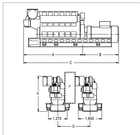
P: Free passage between the engines, width 600 mm and height 2,000 mm
